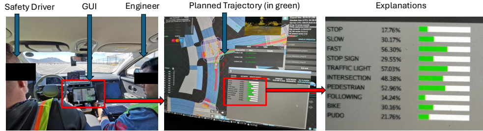
Fig. 2 Deployment setup. A safety driver, a support engineer, and a researcher were present. The safety driver drove the AV manually between road tests, engaged self-driving mode at the start of each test, monitored AV performance during the test, and took over in case of unsafe driving. The support engineer deployed CW-Net and set scenario destinations. The researcher directed testing. The dashboard included a map with overlaid object detections ( s ) from the perception module and the output trajectory ( \hat{\tau} ). Explanations c_i from CW-Net were shown as percentages for easier interpretation [30].
